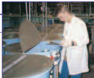
Recording water temperature in a bioassay tank
